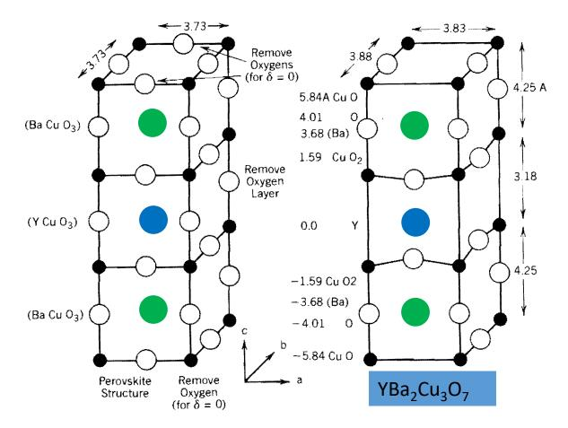
How many oxygen atoms are in the stoichiometric oxygen deficient perovskite unit cell?
